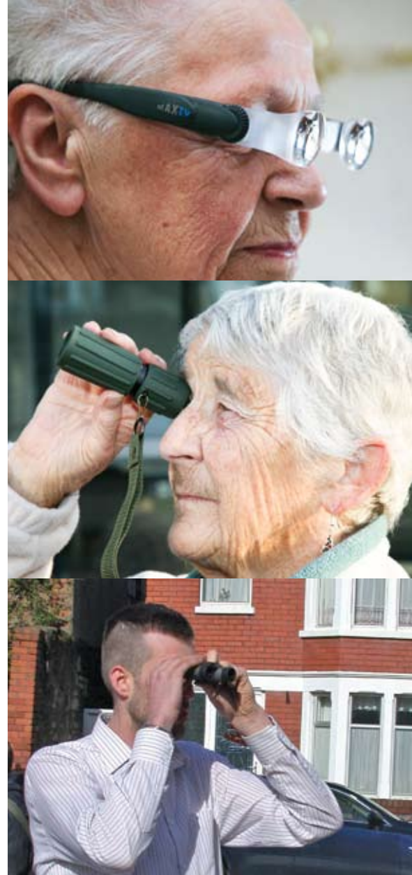
Figure 11: Devices that produce angular magnification: a distance Galilean telescope used for TV viewing, terrestrial telescope and a pair of binoculars.
