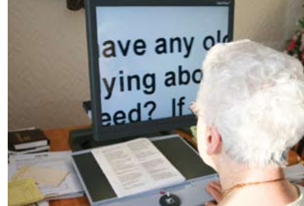
Figure 8: Various models of CCTV are available. The material to be viewed is placed on an X-Y table.
