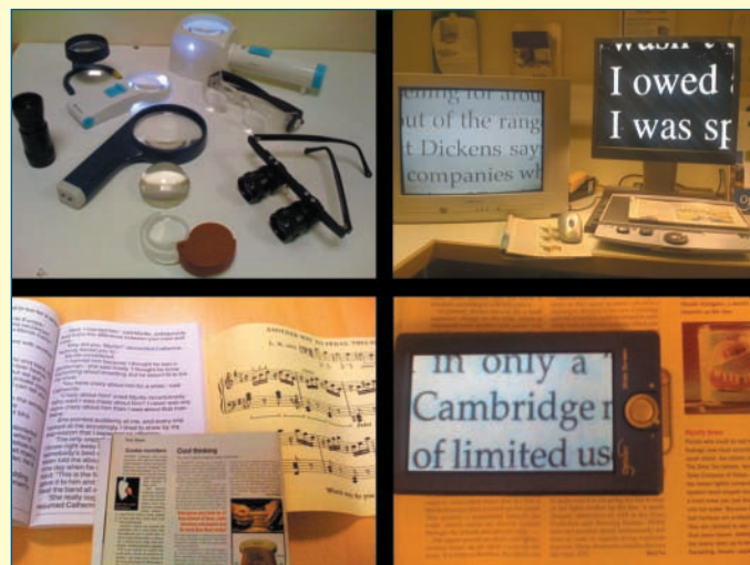
Figure. Top left: A selection of optical magnifiers. Top right: CCTV magnifiers. Bottom left: Samples of normal and giant print. Bottom right: Portable electronic magnifier.
